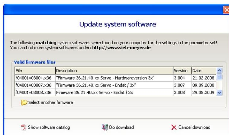
The table lists all firmware and logic files that are available in the installation path of the software *drivemaster2* for the current drive configuration. Select the desired system software.
