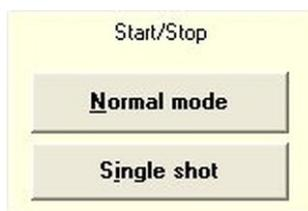
In the "Normal mode" the recording of the selected curves is restarted continuously. The "Single shot" records and displays the curve only once.
