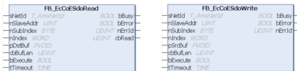
Fig. 27: Function block for reading and writing SDOs
