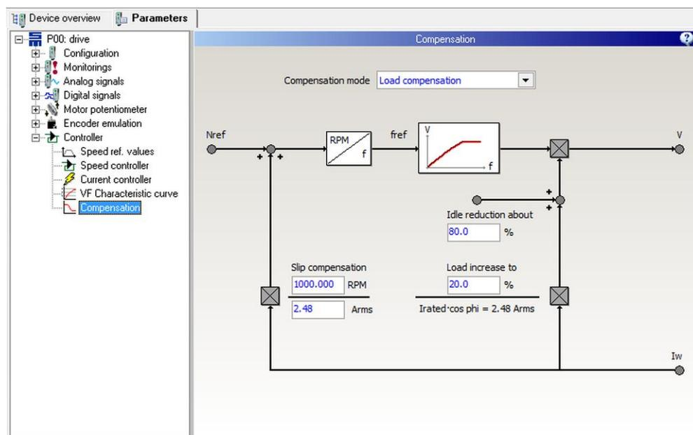
Reduction during no-load operation with overcompensation
