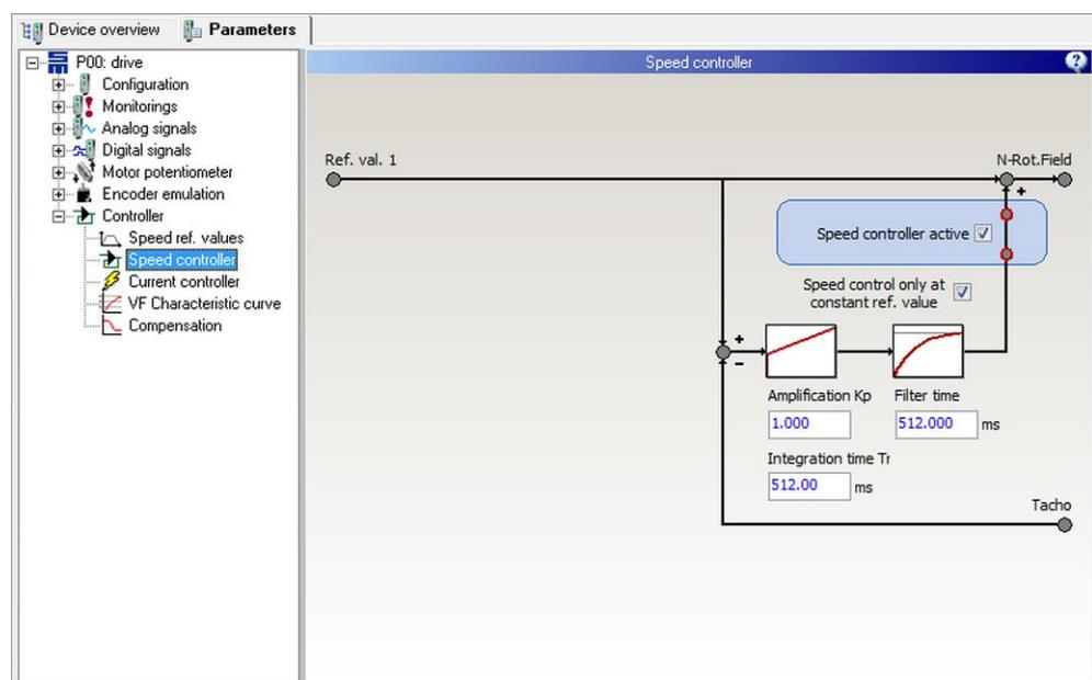
The speed controller is a bypass controller. Due to its structure it can only operate with an amplification ( $K_p$ ) in the range of 0.0 to 1.0.
