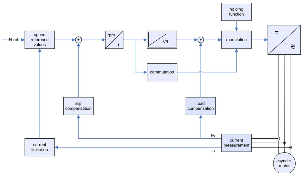
Fig. 1: Structure of the V/f control
