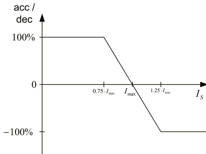
The parameter "Limitation" indicates  $I_{max}$ . The value is taken from the data entered in the parameter wizard and can be changed, if necessary.
