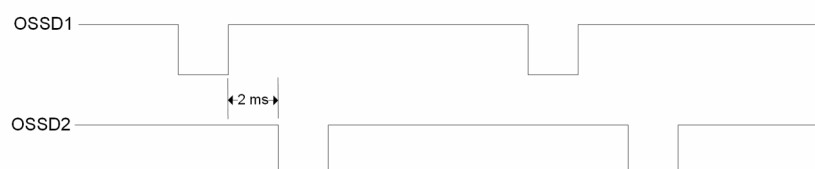
Fig. 14: OSSD test signals
