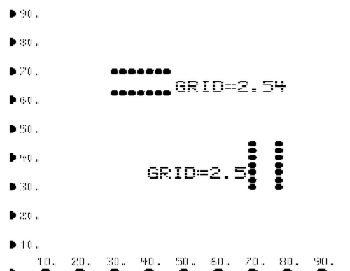
Fig. 14: 2-line drilled rows of holes
