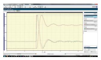
The oscilloscope function allows optimization of the axes in the machine via the drive-setup-tool without additional measuring equipment.
