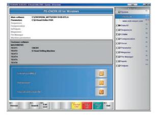
Parameters set the mechanical characteristics of the machine. Functionalities and sequential behavior of the machine are defined in special sequential programs (sequences). This way any machine type can be adapted to the CNC 84.00 by means of the parameters.
