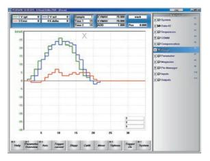
OSCAR is an auxiliary program for optimizing machine movements. By means of the graphic visualization speeds, accelerations, and moving characteristics can be set individually for each axis. This online optimization allows the machine manufacturer to determine the best possible values for a machine and thus achieve considerable improvements in the machine's productivity.
