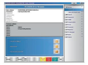
Parameters set the mechanical characteristics of the machine. Functionalities and sequential behavior of the machine are defined in special sequential programs (sequences). This way any machine type can be adapted to the CNC 82.00 by means of the parameters.
